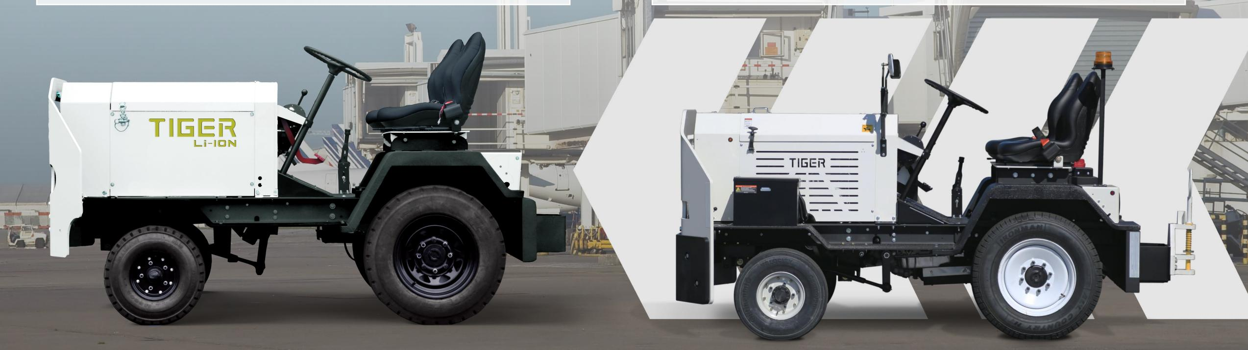
Familiar body-on-frame modular design—steel pieces fastened together, familiar/common design for GSE space
