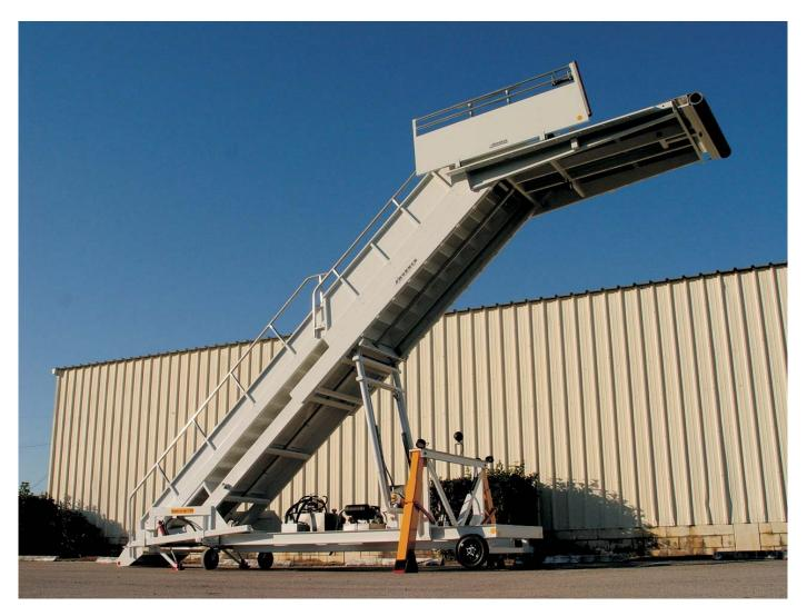
The Phoenix model PAS200 T stair is a towable version of our PAS200 truck mounted passenger stair. The PAS200 T will service commercial and military aircraft with door sill heights between 96" and 208" inches. The model PAS200 T is a two section stair with an "A" frame and four corner stabilizers. The chassis incorporates 4.00 x 8.0" solid tires at the aircraft end and 12" swivel casters at the rear.
